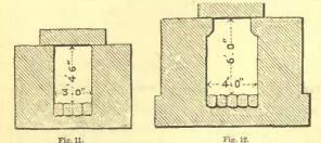
do so. Figs. 11 and 12 are cross sections of medium sized box culverts, the waterway of the onc three feet wide, by four feet six inches high, that
